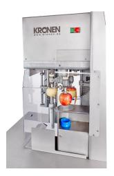
The newly developed apple peeling machine AS 6 for peeling, coring, wedging and slicing apples allows the automatic processing of up to 900 apples per hour
