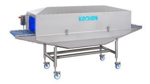
New version: The UVC Disinfection Lock was further developed according to the users' needs (Optional: base with castors)
