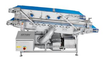
The new version of the belt de-watering system BDS 3000/800 dewaters lettuce, baby leaf and Leaf vegetable and reduces the residual moisture to  $3-8\,\%$ .
